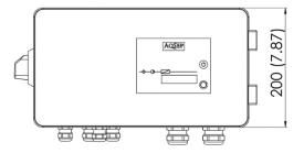
The control box is connected to the sensors on the hydraulic unit via a cable tree of 3 m (9.9 ft.). Separate cables connects the electrical motor and valve.
