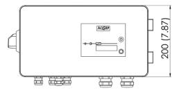
The integrated control box is connected to the sensors via a cable tree. Separate cables connects the electrical motor and valve.
