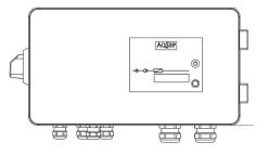
The control box is connected to the sensors on the hydraulic unit via a cable tree of 3 m (9.9 ft.). Separate cables connects the electrical motor and valve.
